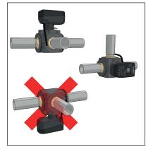
**3.** The actuator can be fitted on the valve body in the two shown positions. It is secured by means of an elastic stainless steel clip.
