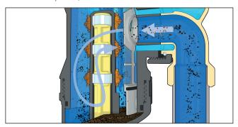
At the device outlet, the water passes through a filter mesh, which retains the residual impurities by mechanically selecting the particles according to their size. The large filter mesh surface with a mesh size of 160µm makes less prone to clogging.
