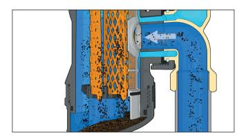
2. The magnets positioned on the central stem capture and trap the ferrous impurities, down to the smallest size.
