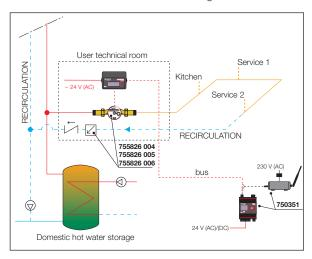
The 755826 00 series kit includes the volume meter with pulse weight 1 l/pulse and the 127 series AUTOFLOW® flow rate regulator for installation to the recirculation pipe.
