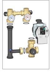
**3.** Unscrew the cap on the right of the mixing valve and screw it on from the opposite side.
