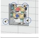
Manually screw the cylindrical guides into the holes in the box.
