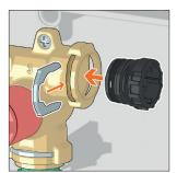
The special connection system does not allow installation errors. The fixing clip only fits into the corresponding groove if the element to be connected is in the correct position.
