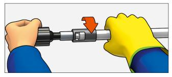
After calibrating the pipe using the relevant calibrator, push the pipe onto the fitting, making sure it reaches the end point. You should look through the windows to make sure the pipe is in the correct position.
