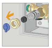
The versions with inspectable main shut-off valves do not have the push-to-open system, and the same knob used for the individual shut-off valves takes its place.
