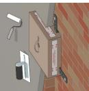
The cover provides a reference for the area to which the surface finish of the wall needs to be applied in order to achieve perfect alignment of the cover
