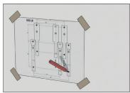
Make the reference marks using the special template and drill the wall.
