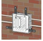
Replace the protection cover before plastering the wall. Use the adjustment screws to make sure the protective mask is flush with the finished wall.
