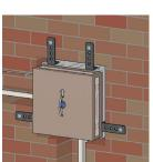
The protection cover protects the inner parts of the box during installation procedures.
