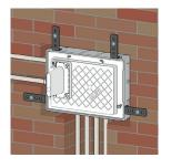
Replace the protection cover before plastering the wall. Use the adjustment screws to make sure the protective mask is flush with the finished wall.
