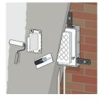
Plaster the wall or lay the tiles right up to the edges of the protective mask.
