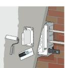
Plaster the wall or lay the tiles right up to the edges of the protective mask.
