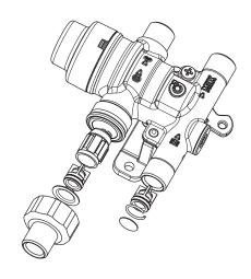
Replacement check valve and strainers for 521201A under sink thermostatic mixing valves.
