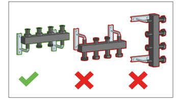
The centre distance of 125 mm makes it compatible with 165 series distribution units, 166 series thermostatic regulation units and 167 series motorised units.
