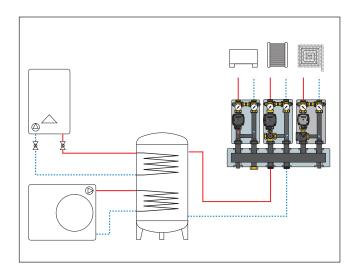
Application diagram, DN 32 Primary connection from right
