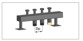
The pressure drop values indicated correspond to a condition of even flow rate distribution across the outlets.
