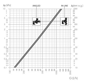
Kv (m³/h) with in-line configuration = 4,2 Kv (m³/h) with angled configuration = 3,9 Maximum recommended flow rate = 1,3 m³/h
