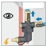
The drain cock can be adjusted by using a wrench (not provided) to loosen the black plastic locking nut.
