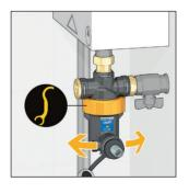
When necessary, it is possible to use the cap with manual air vent to eliminate air inside the strainer.
