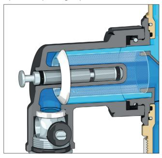
It is possible to drain the impurities without disassembling the body, just by removing the magnet and opening the dedicated cock. Only perform this operation when the system is not in operation.
