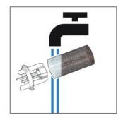
Thoroughly rinse the strainer element under running water, until all impurities have been completely removed.
