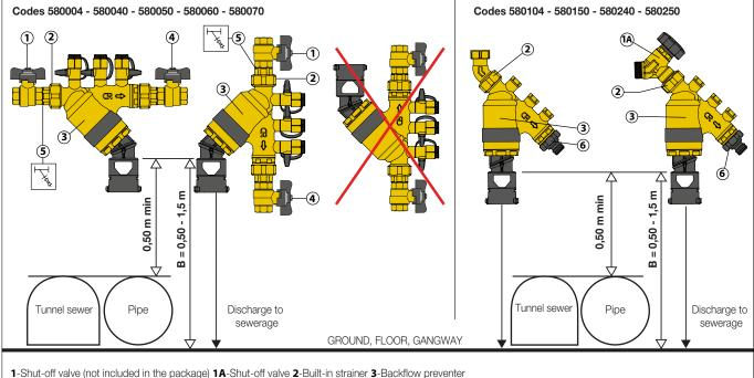
4-Shut-off valve (not included in the package) 5-Optional additional Y-strainer 6-Hose connection
