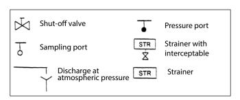
The indications in EN 1717 may be applied to all domestic, industrial/ commercial and non domestic installations connected to the public potable water supply:
