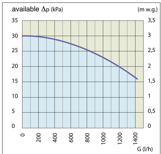
Flow rate range - available head obtainable for modules 700213/14 (setting 20 kPa, on lh side) and 700215/16 (setting 30 kPa, on rh side).
