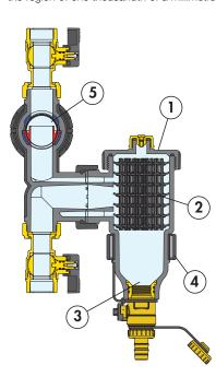
**2.** A replaceable cartridge strainer (5) that mechanically **intercepts** the impurities contained in the thermal medium.
