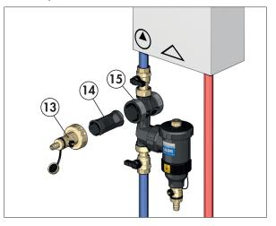
Accessory kit (optional, code F49476) for filling and flushing the circuit consists of a plug with a drain cock (13) and a black coloured element (14) to be fitted in the strainer enclosure (15) to separate the flows.
