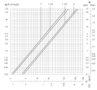
Flow should never exceed standards for pipe size and material.
