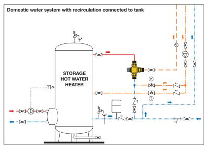
Make sure there is sufficient constant recirculation flow to meet the valve minimum flow requirement, see table on page 4 (4.4 gpm for 1", 1 ½"; 8.8 gpm for 1 ½", 2"). Flow less than minimum may cause valve hunting and fluctuating mixed temperatures.
