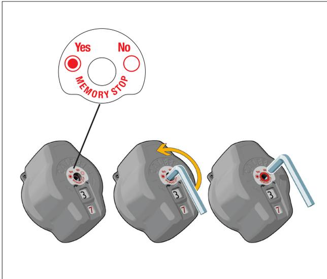
There are two holes on the knob that can be used to seal (5) the setting position to avoid or detect any tampering over time.
