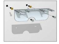
The unit should be applied to the bracket, using the corresponding seats under the hexagonal part of the shut-off valves.
