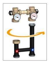
In versions with UPML 25-95 pump, it is necessary to rotate the electronic part of the pump, unscrewing the four screws, as indicated by the arrows, and turning the body anticlockwise by 90°. If this step is not performed, it will not be possible to fit the unit back inside the insulation. In A2L versions with UPM3 Auto L pump no changes are required for the circulation
