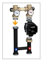
**3.** Position the connecting pipe on the right-hand side, rotating it on its axis by 180°.
