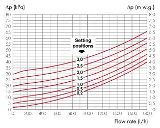
The hydraulic characteristics are calculated while taking account of the ball shut-off valves fitted.
