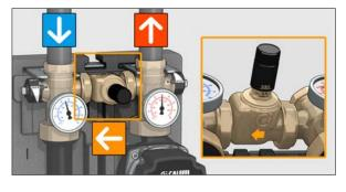
by-pass installation in the version with LH side supply and bottom-up flow (equivalent to RH side supply and top-down flow).
