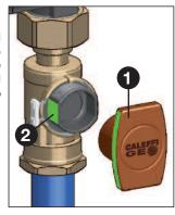
When the control knob is in the vertical position, the ball is open and the medium is flowing (A). When the lever is in the horizontal position the ball is closed: the seats ensure a tight seal and impede the medium flow (B).
