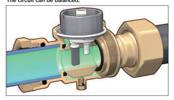
Balancing with the Vortex sensor has many advantages:
