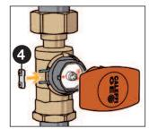
In horizontal installations, liquid above the ball could impede the correct positioning of the sensor in the valve body. For this reason, the valve body is equipped with a cock on the rear (5) to discharge the fluid, contained inside the ball, when this is in the closed position.
