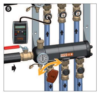
6. This operation must be repeated on subsequent branches to obtain the desired flow rate.
