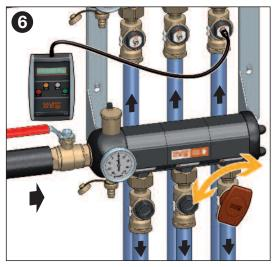
While measuring the flow rate, the sensor creates no significant head losses and therefore causes no significant changes in the actual flow rate.
