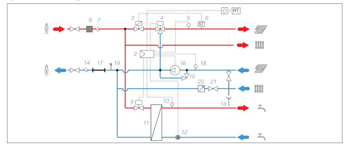
\* N.B. We recommend installing an AUTOFLOW<sup>®</sup> flow rate regulator (20) and a shut-off valve (21) on the circuit serving high temperature heat emitters that must be equipped with temperature control devices.
