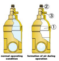
air through the discharge valve (3), during the system filling phase.
