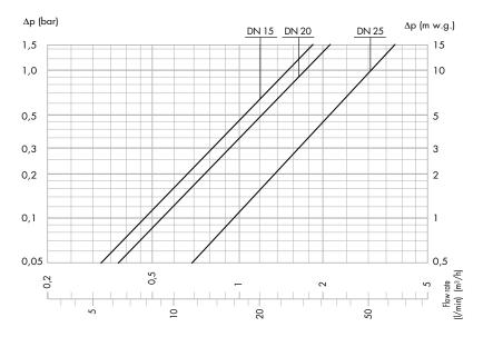
Recommended flow rate values to ensure stable operation with an accuracy of  $\pm$  2 °C
