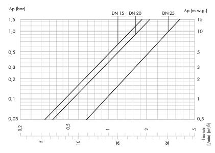
Recommended flow rate values to ensure stable operation with an accuracy of ± 2 °C . . . .
