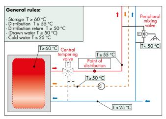
For all these reasons, therefore, a tempering valve must be installed on the hot water storage outlet line, at the inlet point of the distribution system, which is able to:
