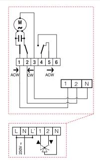
Actuator code 637012 (SM100) with Optimiser® digital climate regulator code 152001
