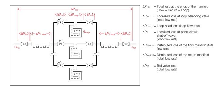
$\Delta P_{\text{Tot.}} = \Delta P_{\text{VR}} + \Delta P_{\text{Loop}} + \Delta P_{\text{VI}} + \Delta P_{\text{Manif. F}} + \Delta P_{\text{Manif. R}} + \Delta P_{\text{VS}} \times 2$  (1.1)
