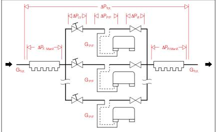
$\Delta P_{LV} = \text{Localised loss in the lockshield valve circuit} \ (P/F circuit flow rate)$
