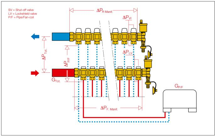
$\Delta P_{\text{Tot.}}$  = Total loss at the ends of the manifold (Flow + Return + Pipe/Fan-coil)
