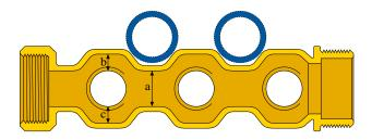
The partial pipe housing in the manifold outline is also helped by the fastening brackets, which are made with an angle that provides a 25 mm offset between the upper and lower manifolds.
