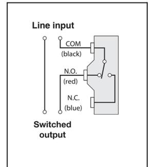
Flow switch used to activate a device when flow stops.
