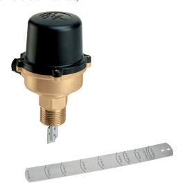
The flow switch should be installed on the pipe with the control rod upright, following the flow direction indicated by the arrow on the cover and on the body exterior.
