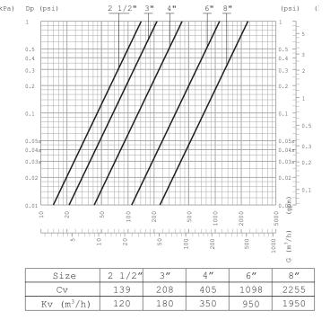
Cv = flow in gal/min for a pressure loss of 1 psi
