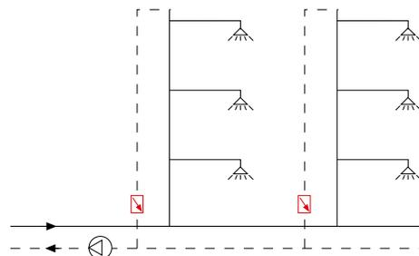
To balance sanitary water distribution circuits
