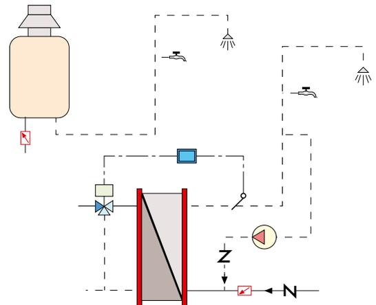
To restrict the hot water delivery flow rate in instantaneous or limited-capacity hot water production systems.
