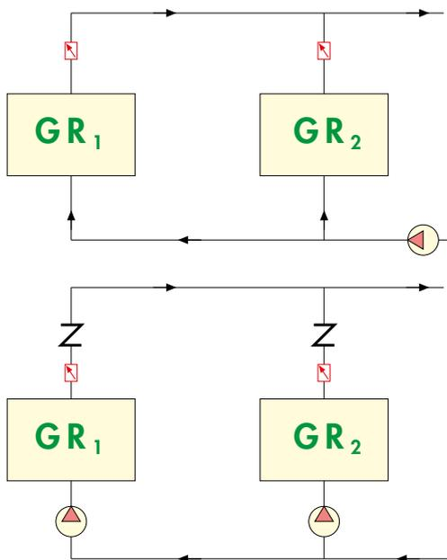
To balance the circuits that serve chiller unit evaporators or condensers.
