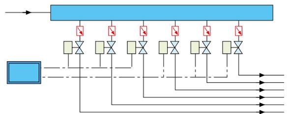
To check the amount of water delivered and balance the various circuits in irrigation systems
