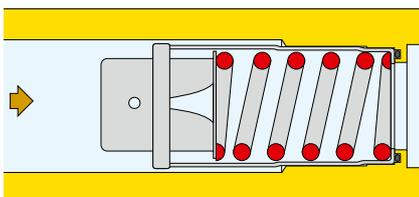
In this case, the piston compresses the spring fully and only leaves the fixed geometry aperture for the medium to pass through. As in the first case above, the piston acts as a fixed regulator. The flow rate through the AUTOFLOW® therefore depends solely on the differential pressure.
