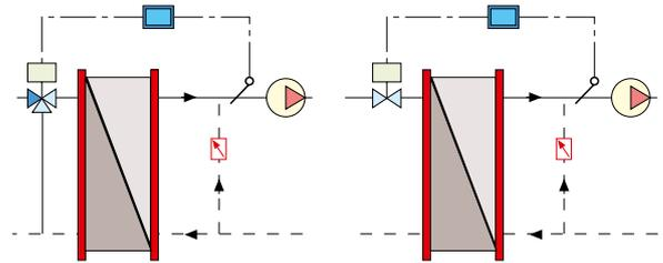
To create flow rate balancing by-passes in heat exchangers.
