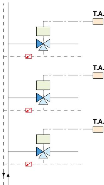
To guarantee the design flow rates (both with open valve and with closed valve) to the various areas in the system.
