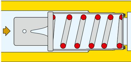
In this case, the regulating piston remains in equilibrium without compressing the spring and gives the fluid the maximum free flow area. In practice, the piston acts as a fixed regulator, and so the flow through the AUTOFLOW® depends solely on the differential pressure.
