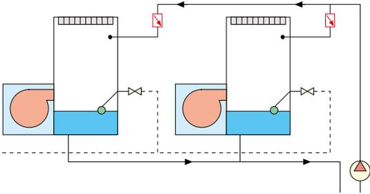
To balance circuits that serve cooling towers
