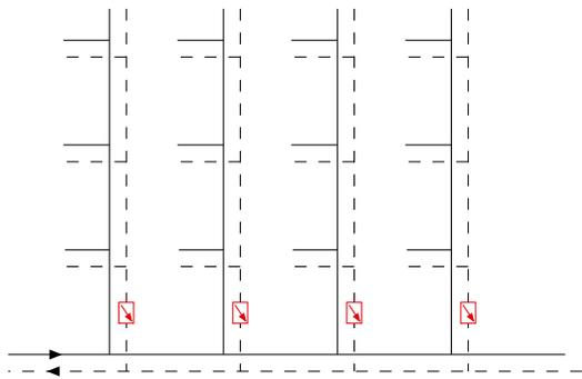
To adjust the flow rate in each column or in each secondary branch of a system.
