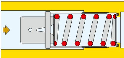
If the differential pressure is within the control range, the piston compresses the spring and gives the medium a free flow area to permit normal flow at the nominal rate for which the AUTOFLOW® is set.
