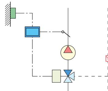
To allow constant flow rates (with the valve in any position) in circuits with traditional climate control.
