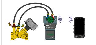
Transmission via Bluetooth® to Smartphone/Tablet with Android® app
