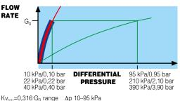
$\begin{array}{ll} {\sf Kv}_{0,01}{=}0,316{\cdot}G_0 \mbox{ range } \Delta p \mbox{ 10-95 kPa} \\ {\sf Kv}_{0,01}{=}0,213{\cdot}G_0 \mbox{ range } \Delta p \mbox{ 22-210 kPa} \\ {\sf Kv}_{0,01}{=}0,158{\cdot}G_0 \mbox{ range } \Delta p \mbox{ 40-390 kPa} \mbox{ where } G_0 = \mbox{ nominal flow rate (l/h)} \end{array}$
