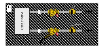
2. Performing a reverse flow operation (the flow of water hits the strainer from the opposite side). The shut-off valve on the flow pipe should be closed before the drain valve is opened.
