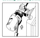
1. Turn the knob to the fully-open position (Pos. 5). With the aid of a screwdriver, unhook the locking nut by pushing it towards the valve body fully.
