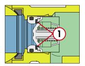
In the event of strong back pressure, the obturator (2) alters the shape of the seal and rests on the actual end point. This solution guarantees optimal device durability.
