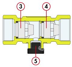
The double check valve may be used, where permitted by current local legislation, as an alternative to the backflow preventer, whenever the water distribution mains has low inlet pressure. The sealing-tightness of the check valve, furthermore, can be tested using the pressure test port in the valve body.
