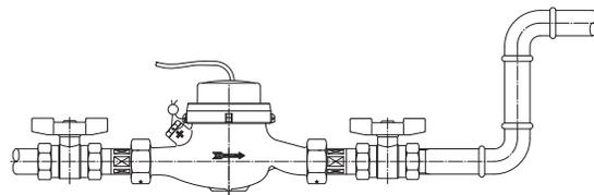
11. With many installations water pipelines serve as earthing for electrical systems. Depending on the actual application an electrical bypass of the volume measuring meter is to be ensured.
