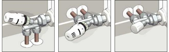
The connection to the pipes does not have a compulsory inlet or outlet direction. To exclude the heating unit, it is necessary to close the knob and, with a 6 mm Allen key, the lockshield valve.
