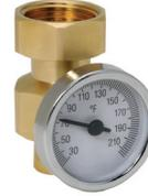
Point of distribution mixed temperature gauge adaptor fits AngleMix™ 520 series mixing valves. Threaded union mounting replaces existing mixed outlet with 3/4" or 1" sweat pipe connection. Removable gauge fits into temperature well. Gauge dial is 2" diameter and scale from 30—210° F.
