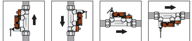
The versatility of the balancing valve means the geothermal manifold can be installed both vertically (wall mounted) and horizontally (in an outdoor well for example).
