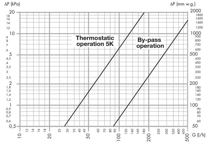
To correctly size the recirculation pump head, add the loss of head of the valve to the loss of head of the most disadvantaged circuit.
