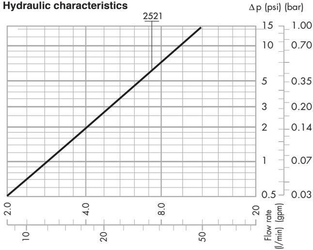
2521 series Cv 3.0 (gpm) (Kv 2.6 (l/min))
