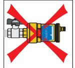
The hygroscopic safety vent operating principle is based on the properties of the cellulose fiber disks forming the retaining cartridge. These disks increase their volume by 50% when they come into contact with water, thus closing the valve. This avoids any damage in the event of water leakage.
