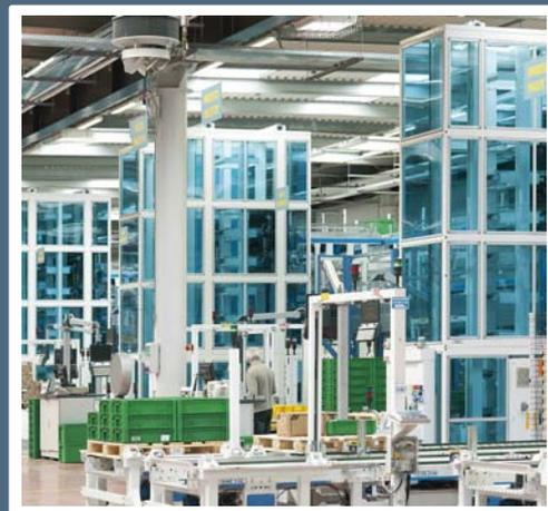
**2.** THE VERTICAL AUTOMATED WAREHOUSE IS COMPRISED OF FREE-STANDING METAL STRUCTURES COMPLETE WITH AUTOMATED HANDLING SYSTEMS. INSIDE THERE ARE TWO SEPARATE ACTIVITY AREAS: A PALLET WAREHOUSE AND A MINILOAD WAREHOUSE FOR PRODUCTS ARRANGED IN CASES. EACH AREA IS ORGANISED INTO 4 CORRIDORS WITH SINGLE-DEPTH SHELVING, EACH OF WHICH IS SERVED BY ITS OWN STACKER CRANE AND POWER RECOVERY SYSTEM, GIVING A TOTAL OF 8 CORRIDORS AND 8 STACKER CRANES WITH INTEGRATED SHUTTLE CARS.
