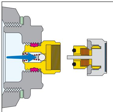
The valve is constructed in such a way that the part which contains the hygroscopic insert replaced can be easily replacement without emptying the radiator. To guarantee the efficient working order of the valve it is necessary to replace the hygroscopic cartridge at least every 36 months (cod. 508100).
