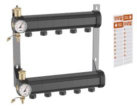
Max. working pressure: 6 bar. Max. system test pressure: 10 bar. Working temperature range: -10-60 °C. Ambient temperature range: -20-60 °C. Medium: water, glycol solutions, saline solutions. Max. percentage of glycol: 50 %. Manifold DN 50. Max. flow rate: 7 m<sup>3</sup>/h. Outlet centre distance: 100 mm. Outlet connections with mechanical seal for 111 series shut-off valves, 112 series balancing valves and 113 series flow meters.
