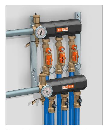
The use of a flow meter makes the system balancing process significantly easier, as the flow rate can be measured and checked at any time and differential pressure gauges or reference charts are not required.
