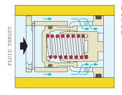
If the differential pressure is within the control FLOW RATE range, the spring-loaded piston is positioned to give the fluid a free flow area permiting regular flow at the **nominal rate** for which the FlowCal is set up.
