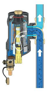
The filter mesh is characterised by various parameters, one the most important being the mesh size (or filtering capacity), which indicates the minimum dimensions of the particles that the filter is able to intercept. Another concerns the filter mesh surface, with a larger surface area guaranteeing a lower degree of fouling.
