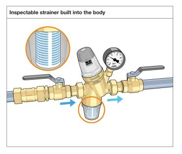
Some pressure reducing valve models are fitted with a high-capacity inspectable strainer, located in a special transparent container. In this way, the pressure reducing valve is a single compact component with protection against impurities that could compromise its operation.
