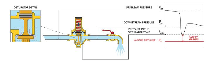
This condition causes the liquid to change to the gaseous phase, forming bubbles that contain vapour.
