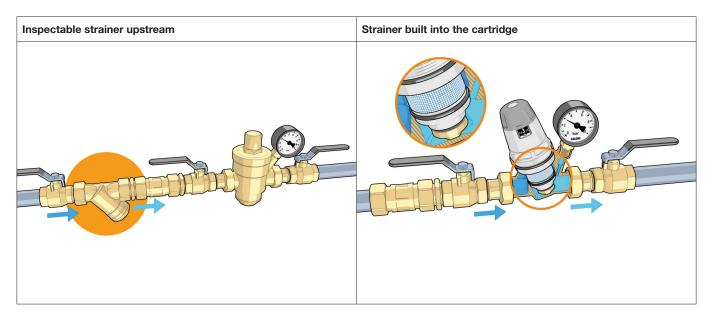
In systems with a high impurity content, it is advisable to install an inspectable strainer upstream of the pressure reducing valve, even if it already has a built-in strainer, in order to perform double filtration.
