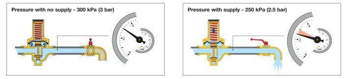
The pressure drop at the design flow rate must always be taken into account when choosing the pressure reducing valve. In addition to verifying the speed, it is always necessary to check that the pressure drop is not too high, otherwise a larger size or a different type of pressure reducing valve must be chosen.
