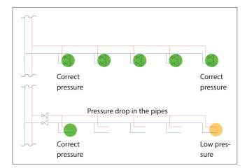
When choosing the correct location for the pressure reducing valves, it is also important to consider the pressure drops due to dynamic effects. In particular, we must prevent the most used areas from subtracting pressure from the farthest areas. When the pipes are undersized and long, the pressure drops due to dynamic effects become considerable, especially in the farthest units. The pressures are lower at these points and may be insufficient for the user.
